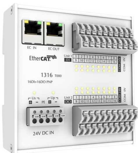
16 x DI, PNP, filter: 3ms 16 x DO, PNP, I max : 0.5A, 24VDC
