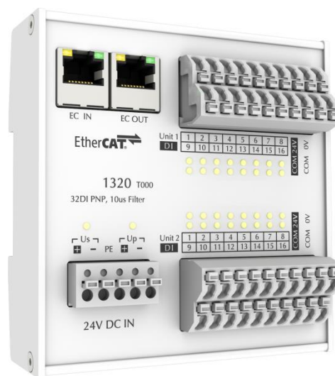
32 x DI, PNP, filter: 10us, 24VDC
